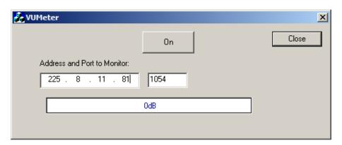
Open VU Meter with the appropriate multicast address and port number entered in the blanks. Turn the program on. Send a test call on the TX or RX port numbers and see if VU Meter indicates digital audio activity. You may open multiple instances of VU Meter to simultaneously monitor TX and RX port numbers.
