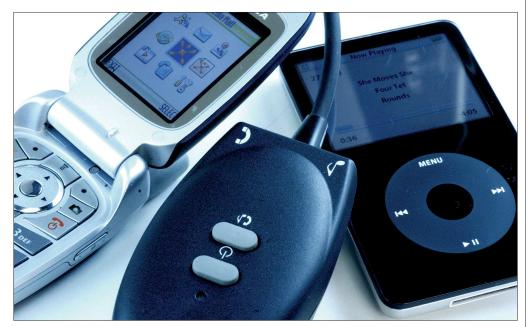
The Telex Stratus 30XT allows you to plug an MP3 player or a cell phone directly into the headset. A flick of the switch mutes the input when communicating with ATC
