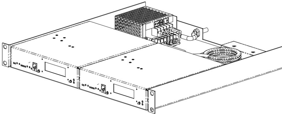
In this solution, Telex IP-223, Dual Network Adaptor Panels provide the functionality required for the parallel operation of two base stations and the back-to-back repeater interface. Operation is such that tone remote control of a particular mutual aid channel by the dispatcher causes both old and new frequency assignments to key and transmit simultaneously.
