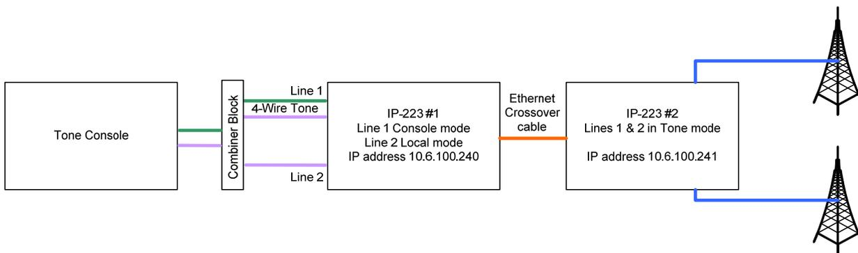
In the reverse direction, subscribers working through either old or new channel assignments would be heard by all parties to a particular mutual aid event. Dispatcher control will be maintained at all times where the dispatcher will have priority over subscriber communications and the capability to enable and disable the repeat function of the various channels – all via standard tone control with no modification to operational procedures in place today.
